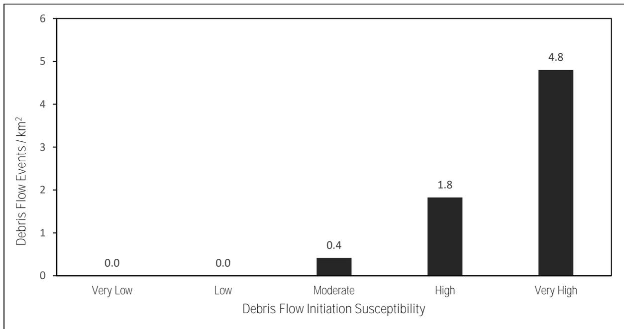
**Figure 3.5** Debris flow areal density versus debris flow initiation susceptibility classification based on aerial photograph inventory at the three test locations.
