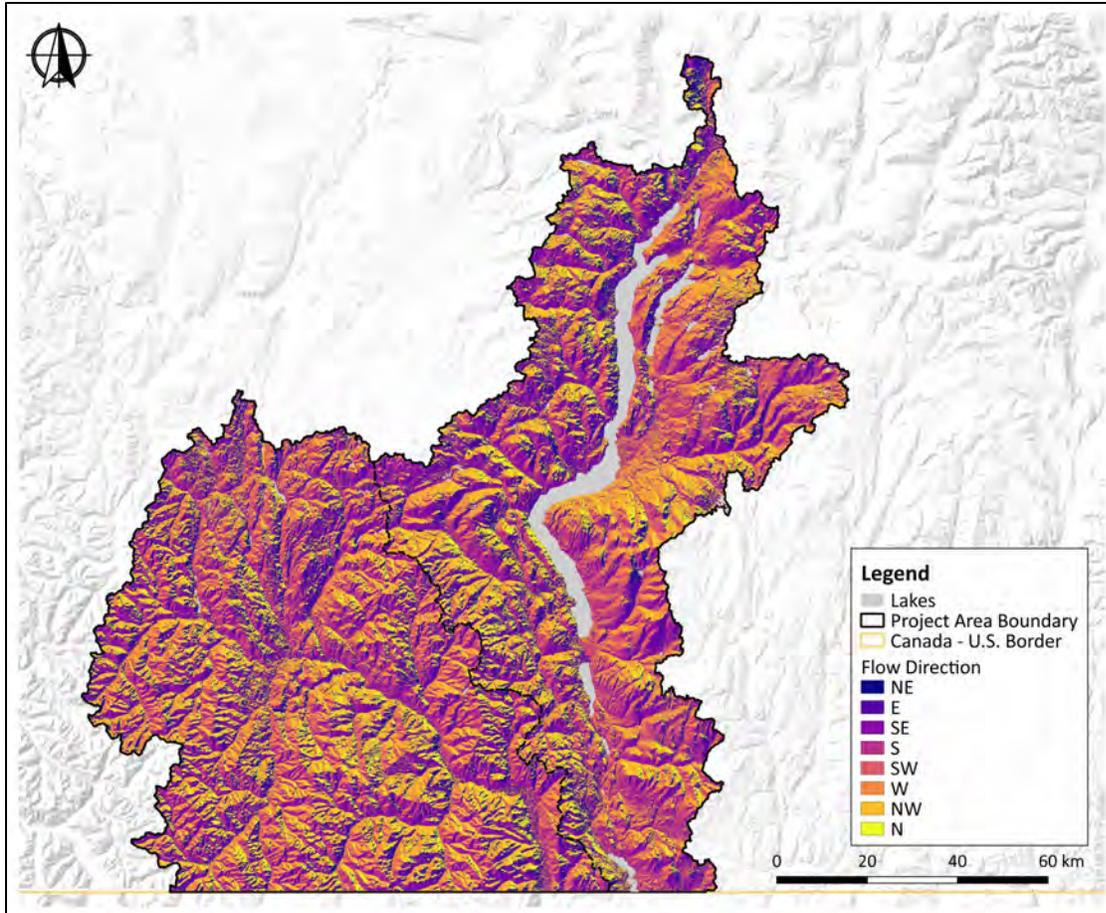
Figure 8: Flow Directions based on the 0.75 arc-second CDEM.
