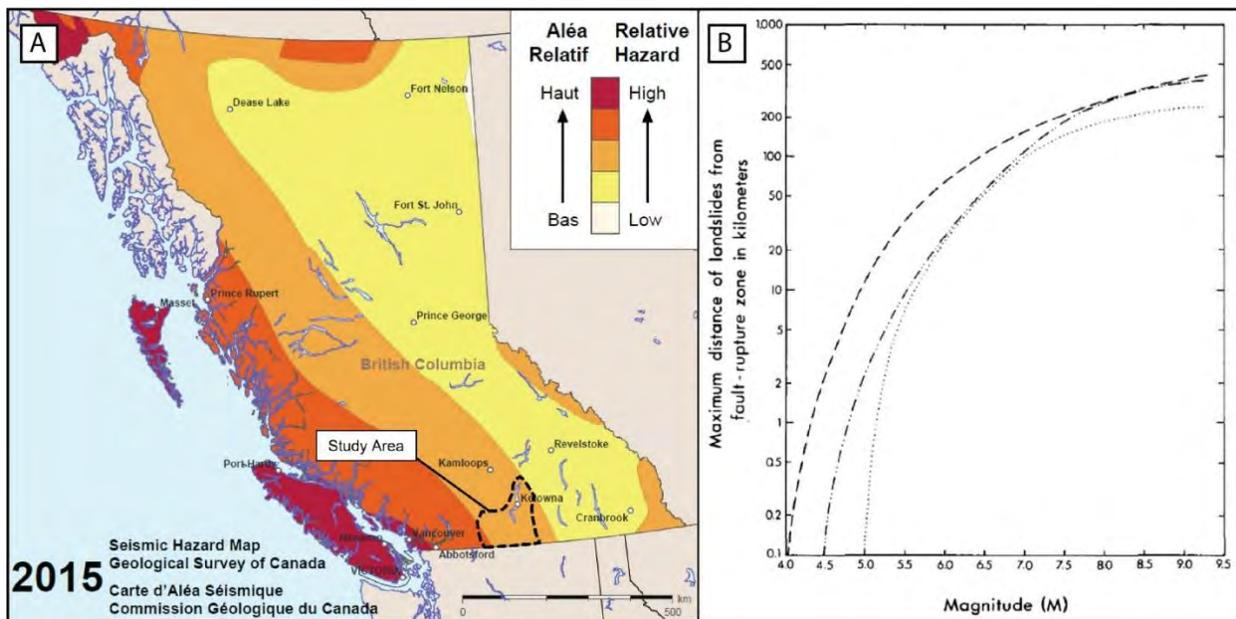
**Figure 4.1 A. Generalized seismic hazard map for British Columbia (NRCAN, 2015) showing the approximate bounds of the study area. B. Relationship between earthquake magnitude and distance at which ground movement may trigger landslides, as determined by Keefer (1984). The dashed line represents disrupted falls and slides, the dashed-double-dotted line represents coherent slides, and the dotted line represents lateral spreads and flows, including debris flows.**
