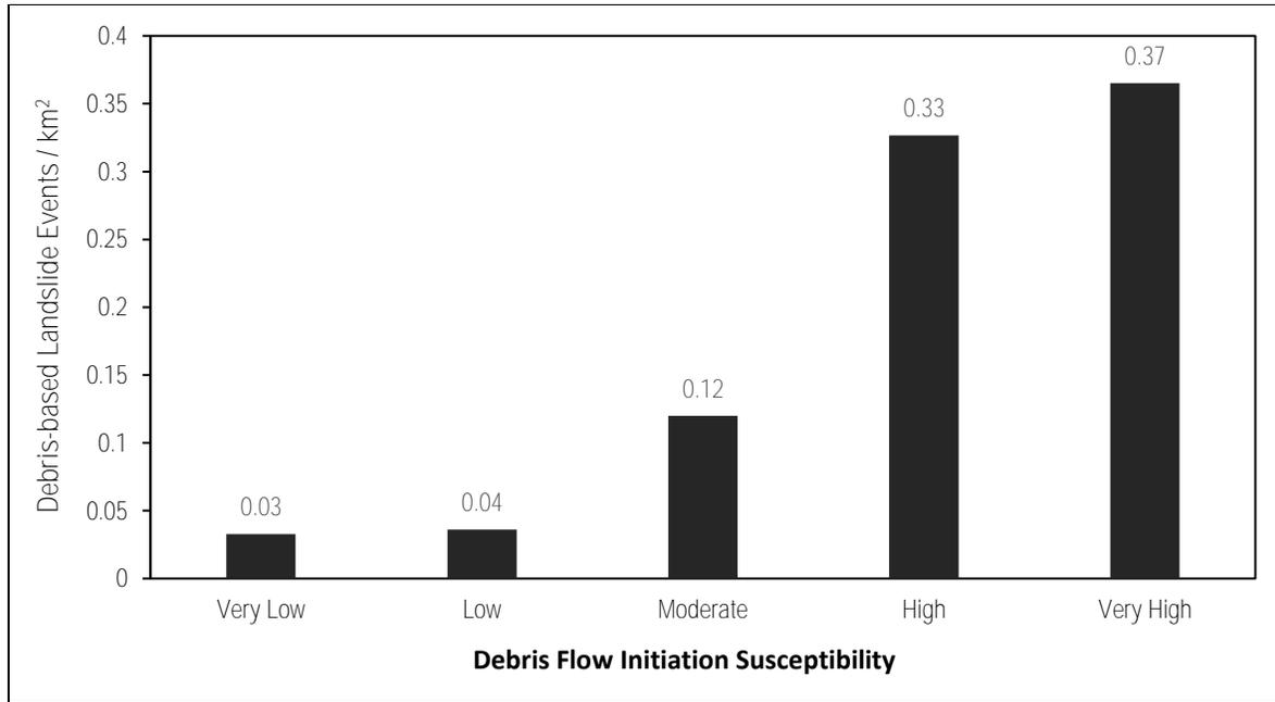
*Figure 3.6 Debris-type landslide density versus debris flow initiation susceptibility classes between Sicamous and Revelstoke, British Columbia. Note that this data set also contains other debris landslide types including debris slides, debris avalanches, debris slumps, and debris floods.*
