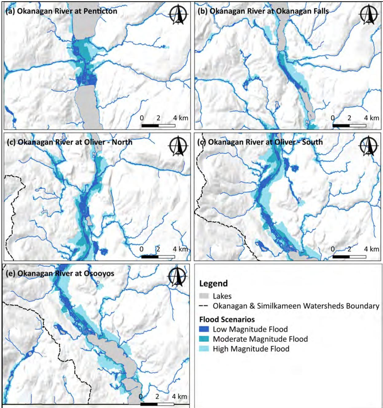
Figure 15: Low, moderate, and high magnitude flood scenarios for the Okanagan River, as determined by the GFA analysis.
