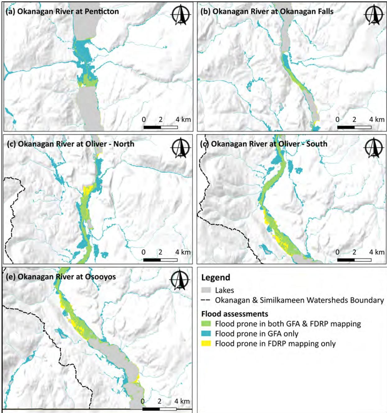
Figure 11: Comparison of flood prone areas identified by the GFA and the FDRP floodplain mapping for the Okanagan River.
