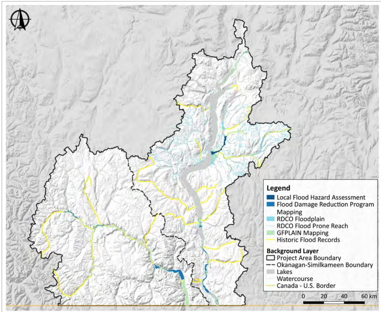
Figure 2: Extents of existing flood hazard mapping, information sources, and analyses in the Okanagan-Similkameen region. Acronyms appearing in the legend are explained in the following sections.
