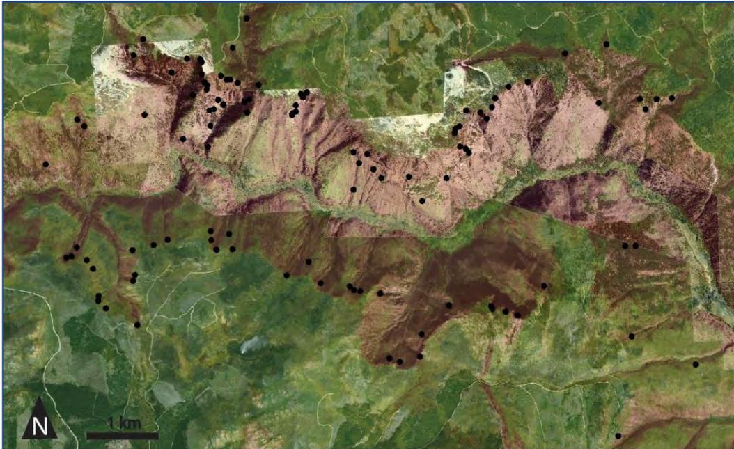
*Figure 3.2 Manually delineated debris flow initiation zones (points) overlain on the debris flow hazard model at test area 2 within Fintry Provincial Park, British Columbia. The test area location is shown in Figure 1.1.*
