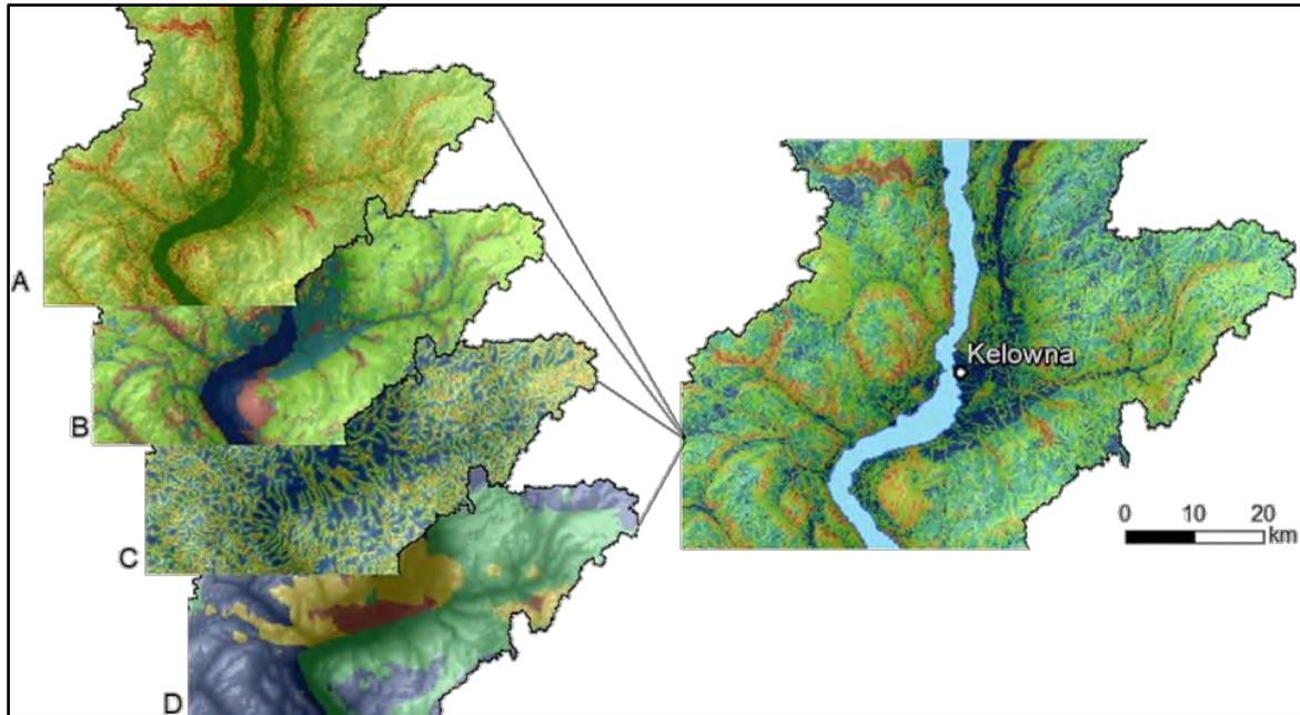
**Figure 2.1 Debris flow initiation susceptibility model inputs (left): A. Slope gradient B. Surficial material C. Distance to drainage D. Bedrock geology. These inputs are combined to create the debris flow initiation susceptibility model (right).**
