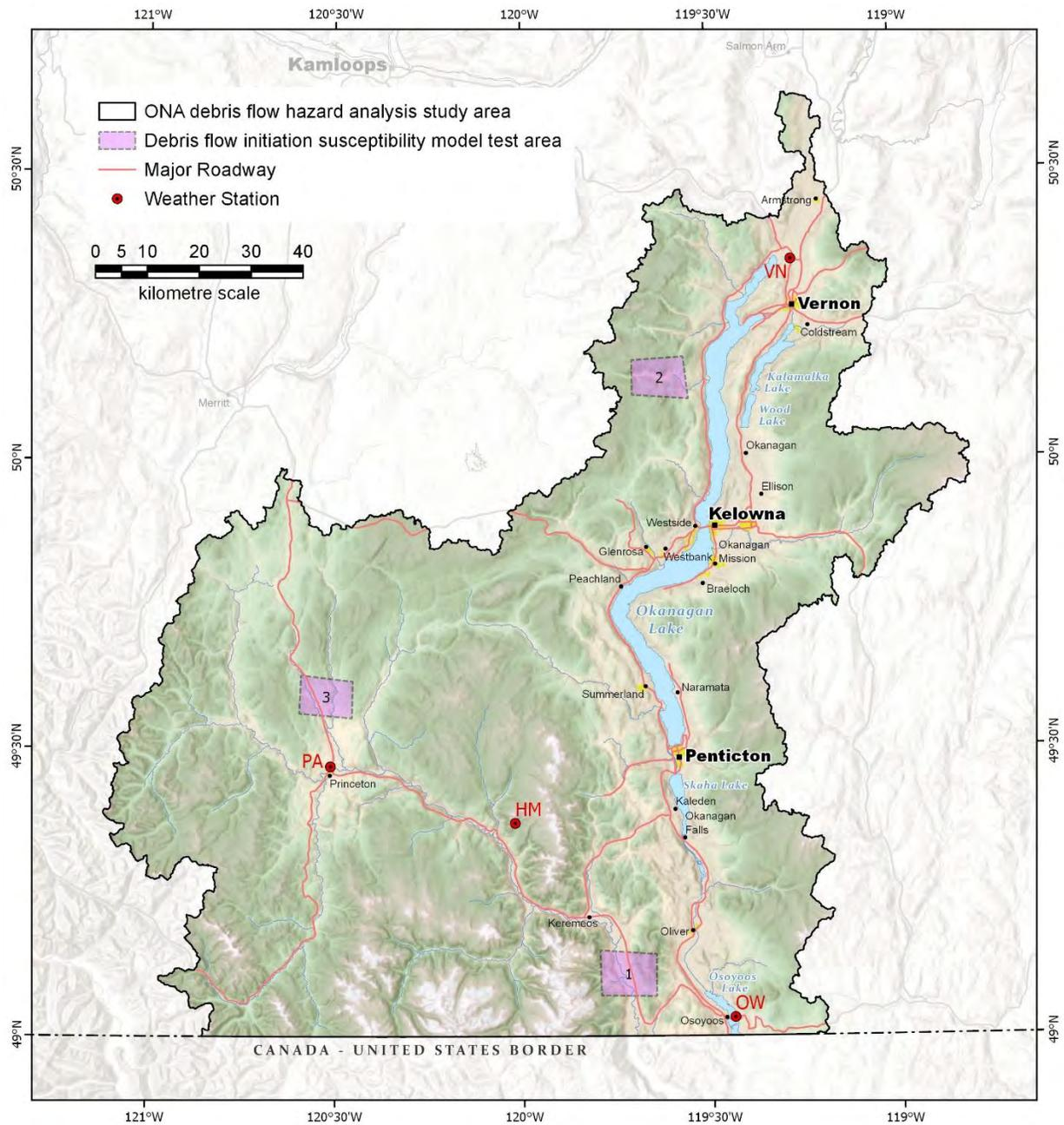
**Figure 1.1** ONA debris flow hazard analysis study area. Locations of weather stations (PA – Princeton A, HM – Hedley Mine, OW – Osoyoos West, VN – Vernon North) shown in Figure 1.2. Debris flow initiation susceptibility model test areas were used to map debris flow initiation sites shown in Figures 3.1, 3.2, and 3.3.
