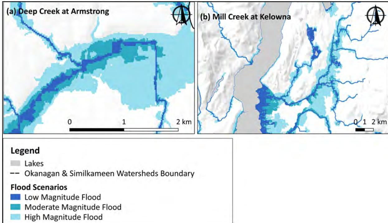
Figure 16: Low, moderate and high magnitude flood scenarios for Deep Creek and Mill Creek, as determined by the GFA analysis.
