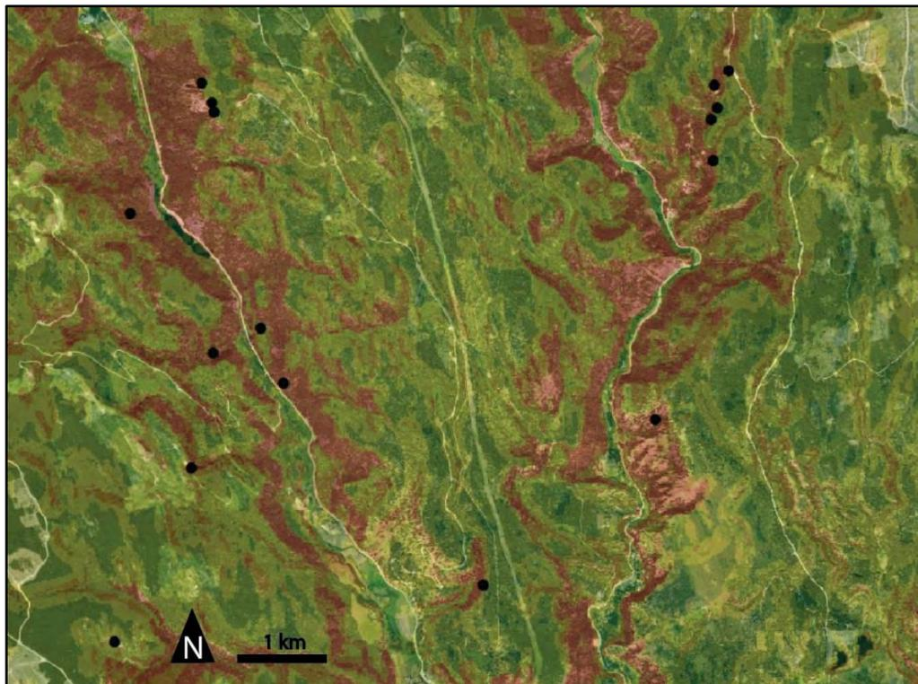
*Figure 3.3 Manually delineated debris flow initiation zones (points) overlain on the debris flow hazard model at test site 3, 15 km north of Princeton, British Columbia. The test area location is shown in Figure 1.1.*
