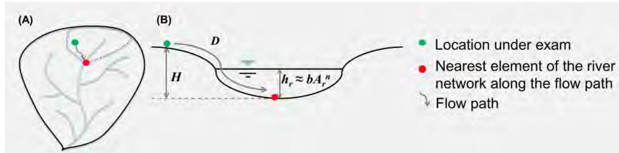
Figure 6: Schematic for the Geomorphic Flood Index (GFI), calculated as  $GFI = \ln(h_r/H)$ . (A) Representation in watershed. (B) Conceptual model of river cross section. Figure by (Samela *et al.*, 2017); creative commons license CC BY-NC-SA.
