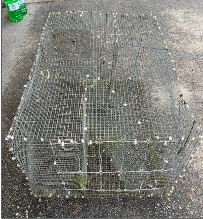
Figure 5. Example of an “N” Trap used for young-of-year Northern Pike sampling. Photo by Ross Zeleznik, Okanagan Nation Alliance.
