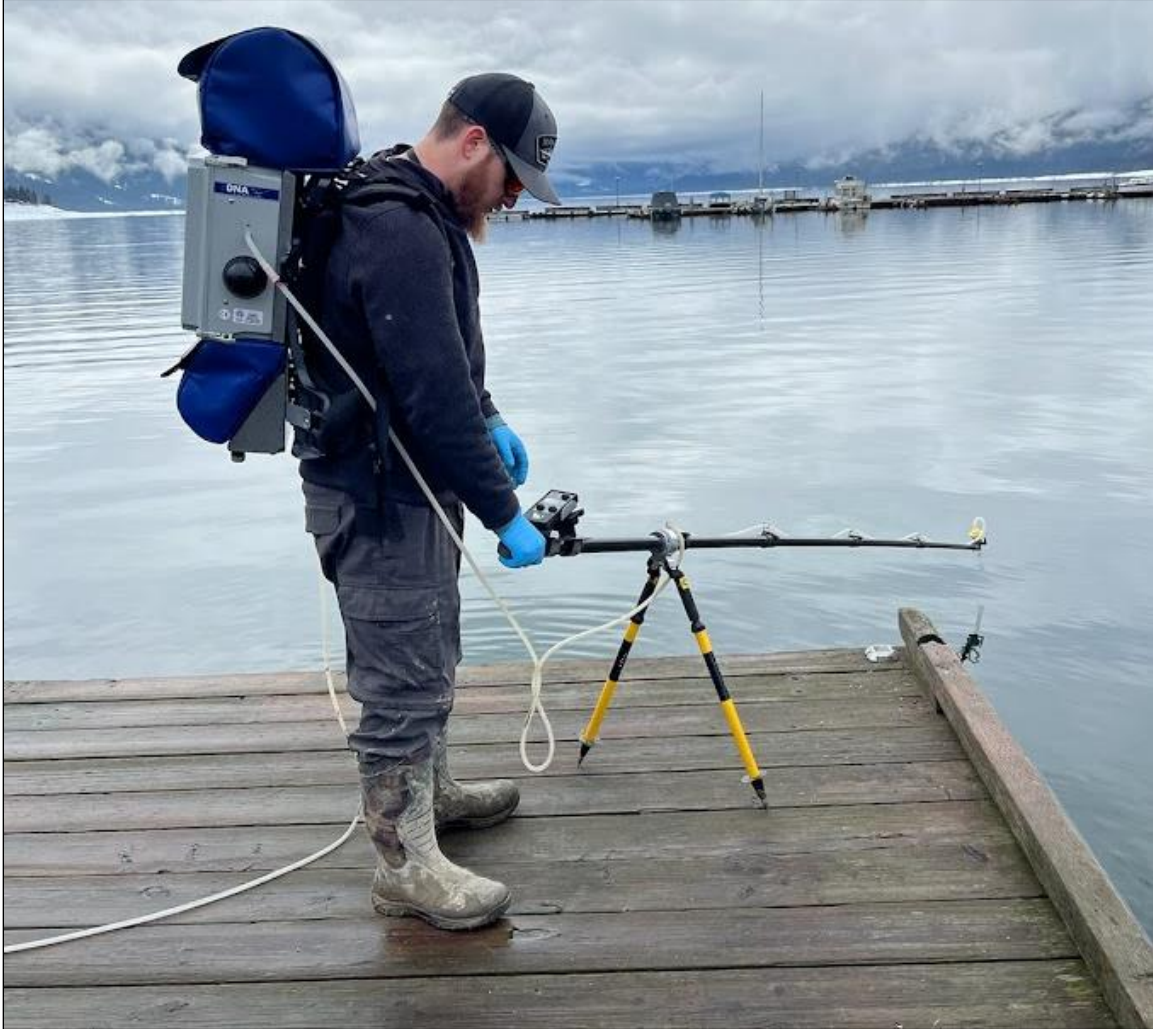
Figure 6. Smith-Root eDNA backpack sampler used to detect presence of Northern Pike in the Columbia River Watershed. Photo by Shelley Hackett, Okanagan Nation Alliance.
