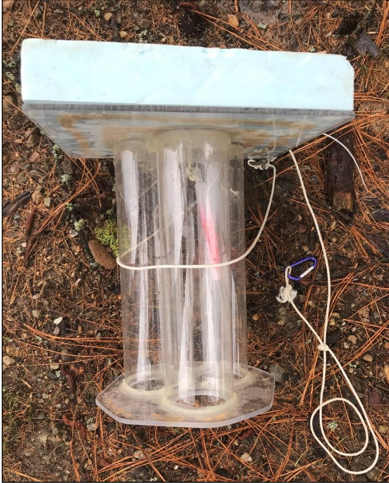
Figure 4. Quatrefoil light trap used to sample for young-of-year Northern Pike in 2020.
