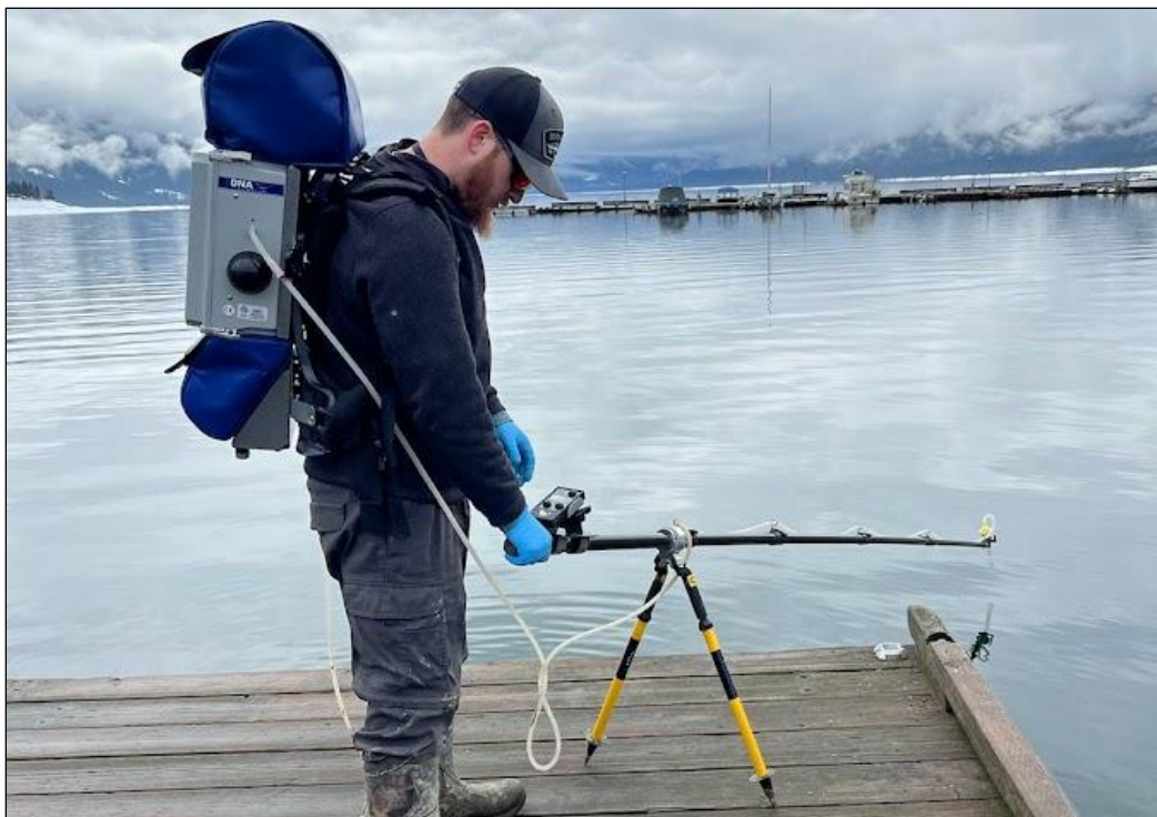
Figure 5. Smith-Root eDNA backpack sampler used to detect presence of northern pike in the Columbia River Basin. Photo by Shelley Hackett, Okanagan Nation Alliance.
